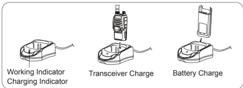
2. Plug the Li-ion battery or the transceiver installed with Li-ion battery into the matched charger.
